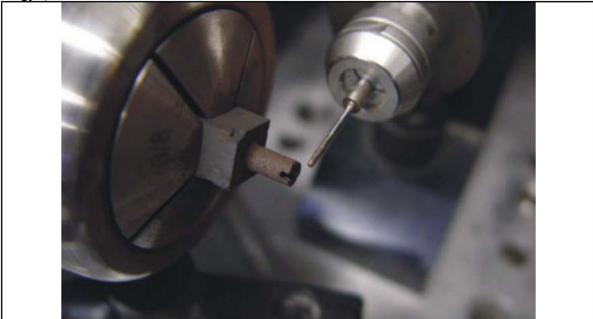
Fig. 4: A thermocouple slot being cut into a lanthanum chromite sleeve on the automated lathe. The hole has already been drilled in the middle and the outside turned down to the correct diameter. After this, the sleeve will be parted off and is ready to use. All these steps are done automatically; the ceramic can also advance for the next sleeve automatically thanks to a compressed air advancer designed by Brian Nagy and Zoltan Farkas.
