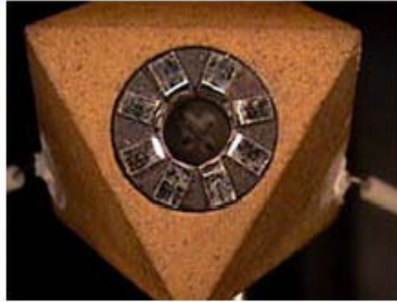
Fig. 3: Rhenium furnace rectangle (left) about 8 mm across, cut by the wire EDM technique, with narrow slits and two thermocouple slots. The rhenium is wrapped and placed into an 8/3 assembly (right – shown with a conventional octahedron from Mino Yogyo).
