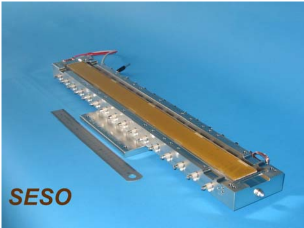
Figure 2: New focusing mirror for high pressure experiments. The mirror is 10 cm long and 1 cm wide. The ray intensity is increased by a factor of 10. Courtesy of the Advanced Photon Source.
