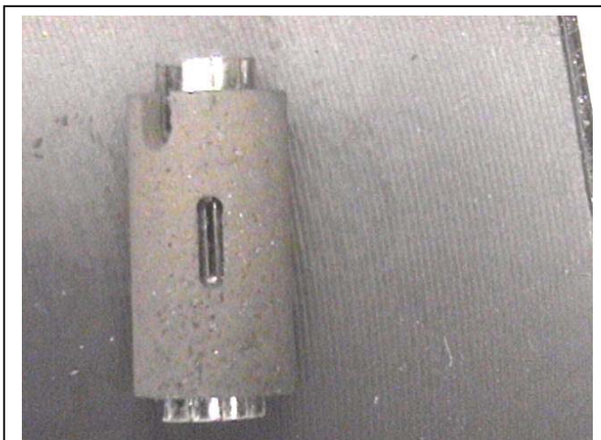
Figure 2. LaCrO 3 sleeve with thermocouple slots and x-ray window cut on the COMPRES automated lathe. The slit in the rhenium furnace from Figure 1 is also visible.
