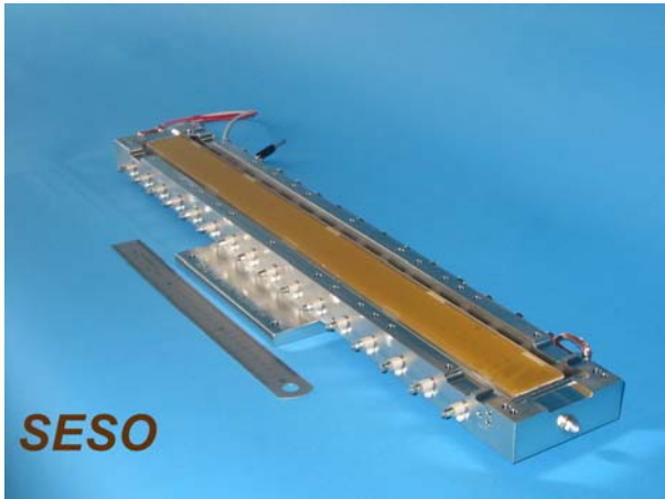
Figure 2: New focusing mirror for high pressure experiments. The mirror is 10 cm long and 1 cm wide, providing a 100-fold increase in x-ray intensity. Photo courtesy of [unclear].
