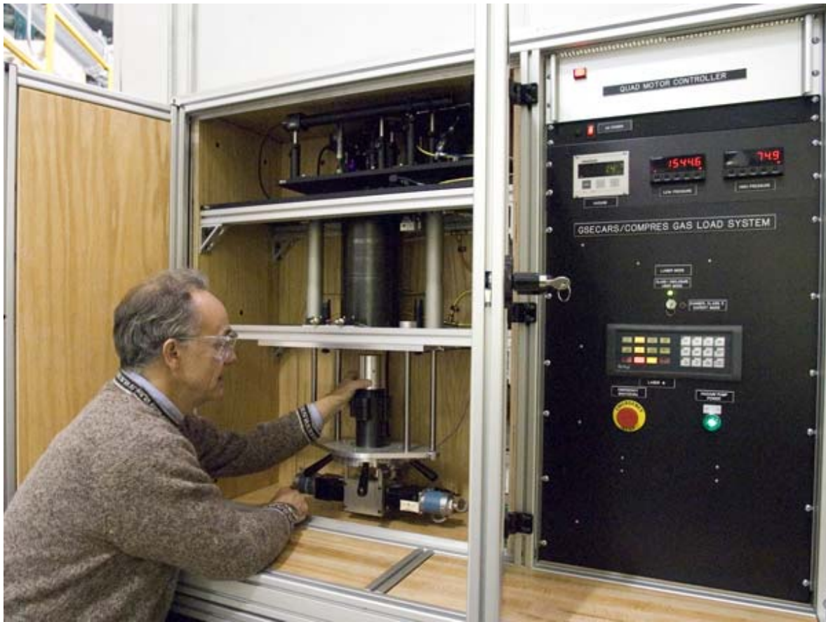
Fig. 1. Mark Rivers and new gas-loading system for diamond-anvil cells constructed at the GSECARS beamlines at the Advanced Photon Source with support from COMPRES and GSECARS.
