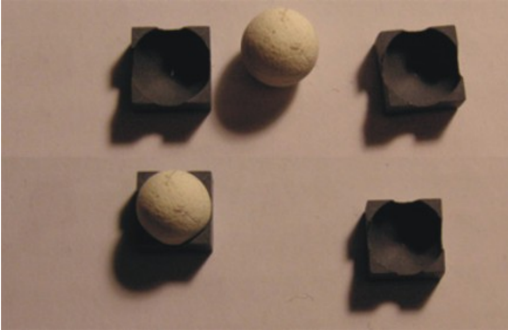
Fig. 7. Mullite spheres and seats made by our project (19)
