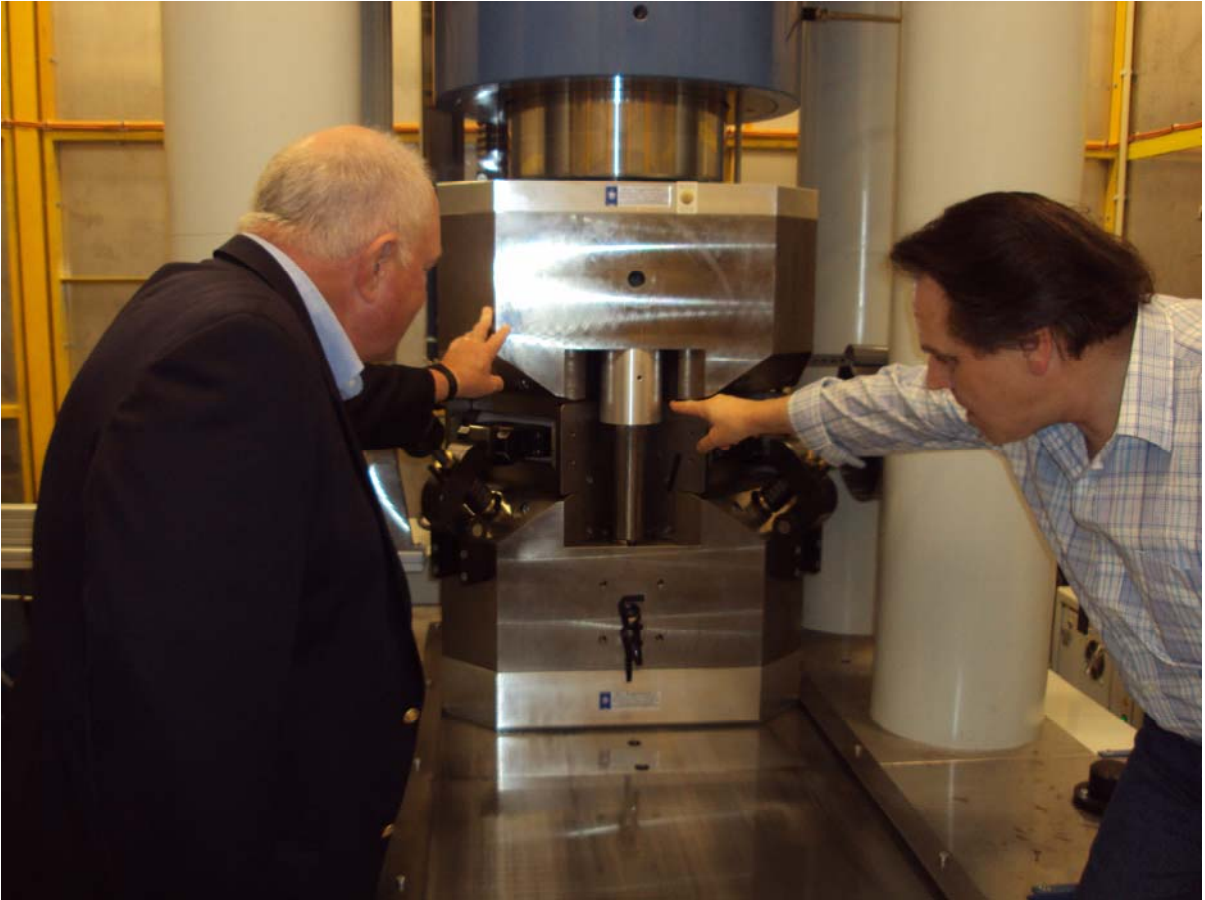
Figure 8. Hans-Joachim Mueller showing Bob Liebermann to the DIA-type guideblock in the MAX-200X at the DESY Synchrotron in Hamburg, Germany in September 2009.
