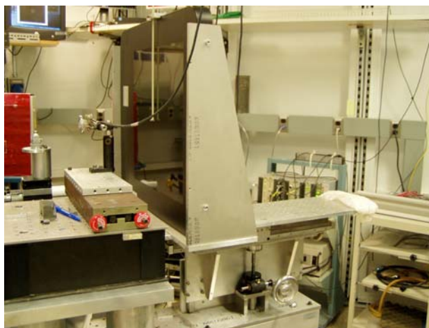
Figure 3. PE Flat Panel detector mounted on newly designed detector bench.
