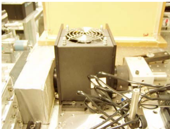
Fig. 7. IPG fiber laser (1066nm, 100W)
