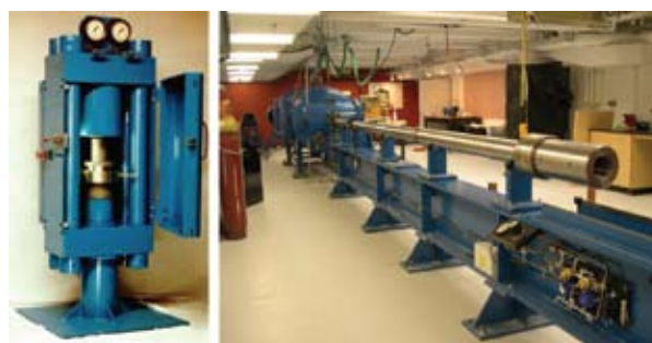
Figure 1.4. (left) Piston-cylinder-type apparatus. The height is about 1.5 m and the sample, which is typically a few millimeters on a side, is contained within the central gold-colored column. These apparatuses have typical pressure limits that correspond to 100-km depth in the planet, and have been extensively used to constrain magma chemistries and fluid-rock interactions in the uppermost region of the planet. Image courtesy of Rockland Research. (right) A shock wave gun. The gun's length is ~15 m. In effect, this piece of equipment is a cannon that fires a gas-driven projectile into a sample, and the sample is intensively monitored while it is compressed to high pressures during the shock event. Pressures that span Earth's entirety can be accessed by shock-wave techniques. Photo courtesy of S. Stewart, Harvard University.
