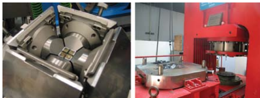
Figure 6.1. (left) View from above, with top anvil assembly removed, of a multi-anvil press. The sample assembly is sitting in the square region between the four visible hydraulically driven anvils (a fifth provides the base of the central square). Scale across the picture is approximately 0.7 m. Photo courtesy of Y. Wang, Advanced Photon Source. (right) Representative hydraulic press in which multi-anvil assemblies are compressed. The bottom anvil assembly (steel-colored object on left) has been slid out of the press. This is a 2000-ton Sumitomo Industries Press currently installed at Stony Brook University. Photo courtesy of R. Liebermann, Stony Brook University.
