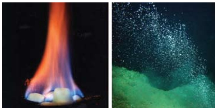
Figure 7.5. (left) Combustion of methane-ice clathrates. Photo courtesy of the Naval Research Laboratory. (right) Release of methane bubbles from the Hakon Mosby mud volcano at 1250-m depth in the Barents Sea. At this location, methane clathrates have been found to exist within 2 m of the seafloor. Reprinted from Figure 2a in Sauter et al. (2006), copyright 2006, with permission from Elsevier.
