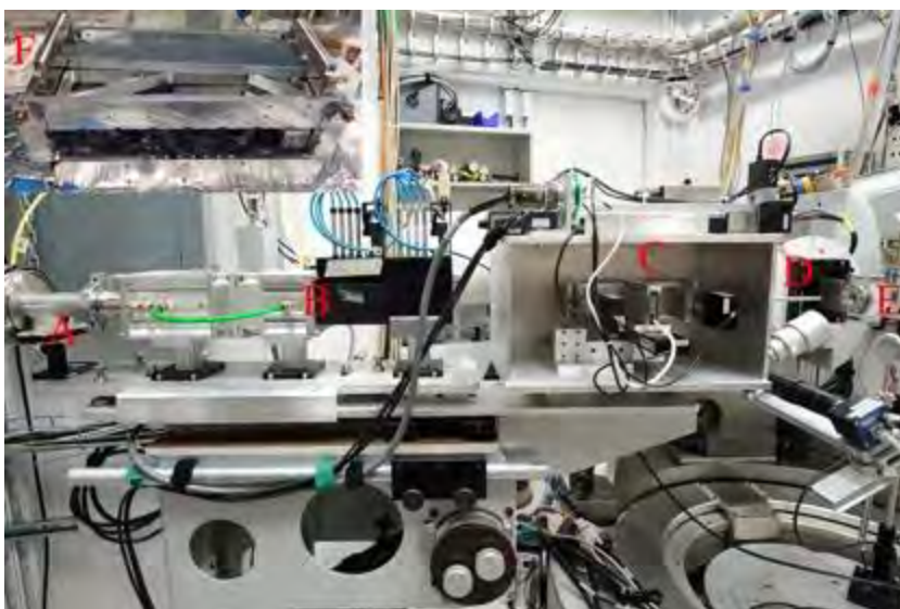
Fig. 3: Major X-ray optics in 13-BM-C for high pressure single crystal diffraction. A: Shielded beam pipe. B: Bench shutter and filter set. C: Horizontal K-B mirror enclosure. D: Motorized cleanup slit. E: Diamond anvil cell. F (inset): Upgraded horizontal K-B mirror.
