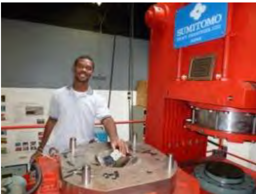
Fig. 5. Brandon Rhymer with 2000 ton uniaxial split sphere apparatus in the Stony Brook High Pressure Laboratory
