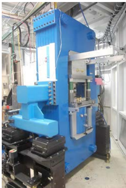
Fig. 6: The new 1000-ton press at beamline X17B2
